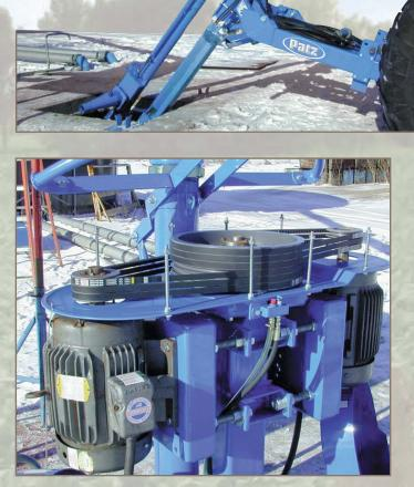
Twin motor belt drive system is easier on the upper drive shaft and bearings. (Guard removed for photo.)
